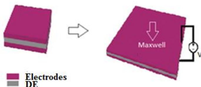
Figure 1. Working principle of dielectric elastomer actuator.
